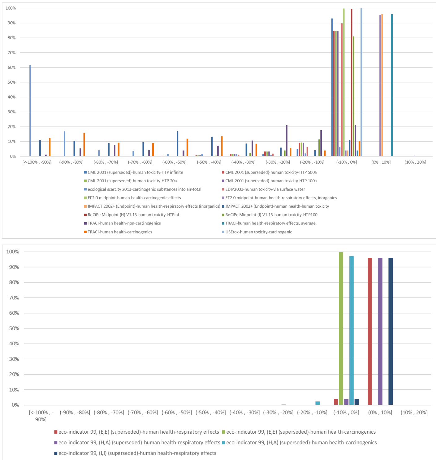
Figure 4. Changes in results obtained for human health categories between v3.7 and v3.7.1 in the APOS system model. As described in the text, indicators were selected to capture the change in results under this category. The vertical axis represents the proportion of datasets affected by a change in scores between v3.7 and v3.7.1 (the ecoinvent database contains more than 19'000 datasets in this system model, 10% of the database covers more than 1'900 datasets). The horizontal axis shows the changes in scores between v3.7 and v3.7.1, grouped in intervals.
